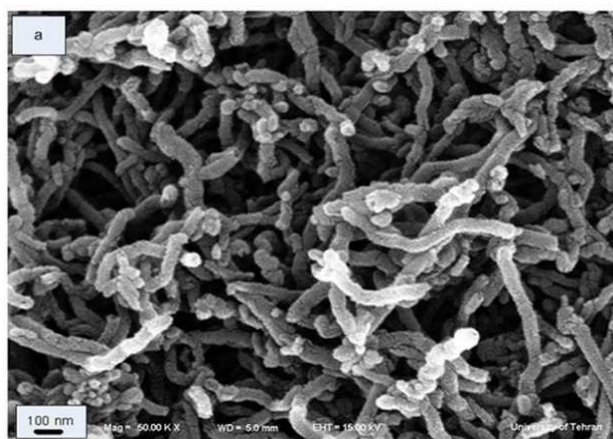
Figure 3. FE-SEM image of MWCNTs: a) before and b) after precipitation of silver nanoparticles
